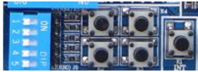
Figure 4-30 Independent Key and External Interrupt Module
